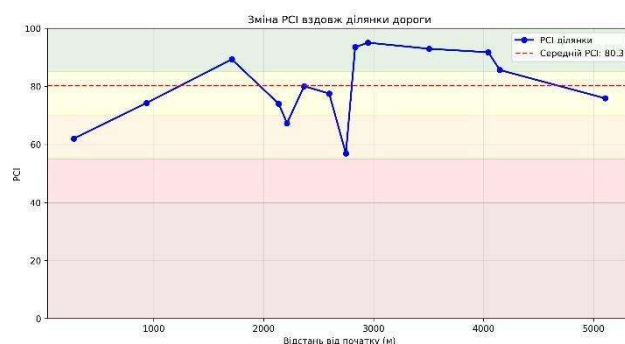
Fig. 4. Example of PCI calculation — road surface damage assessment according to standard [7]
