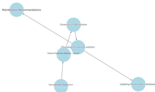
Fig. 1. Adaptation of CBR Decisions Considering Probabilistic Analysis of SPP Equipment Failures
