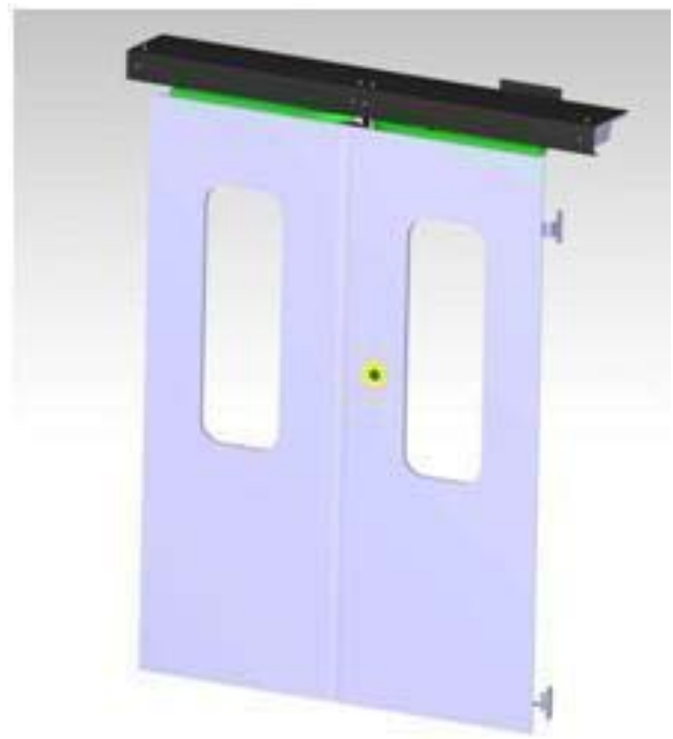
Fig. 1. Designed door system – external view
