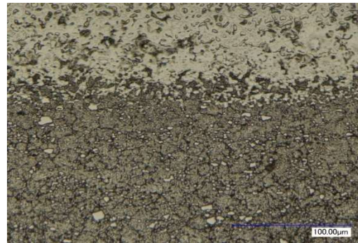
Fig. 4. Microstructure of the surface layer of P6M5K5 steel after electron beam treatment: q = 1.2 \cdot 10^4 \text{ W/cm}^2 ( V = 11 \text{ mm/s} ); x600
