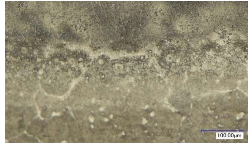
Fig. 3. Microstructure of the surface layer of P18 steel after electron beam treatment with melting: q = 1.35 \cdot 10^4 \text{ W/cm}^2 ( V = 11 \text{ mm/s} ); x600
