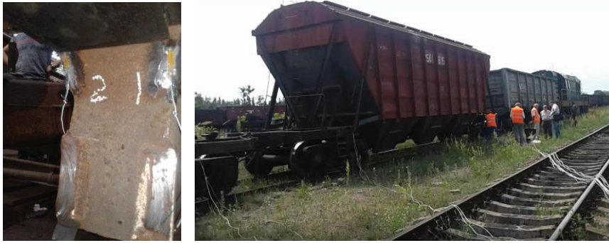
Fig. 3 Scheme of strain gages and the general view of the car
