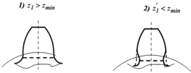
Fig. 1.33. Tooth undercut in gear cutters manufacturing
