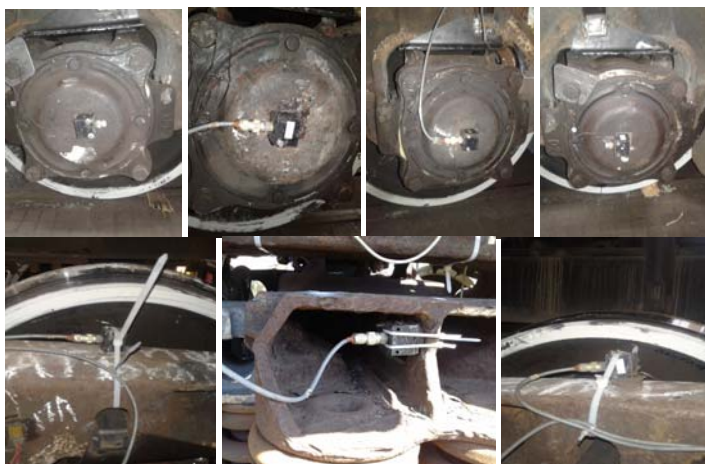
Fig. 3.38. Places of installation of accelerometers in tests
