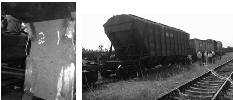
Fig. 3.28. Scheme of strain gages and the general view of the car
