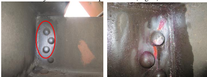
Fig. 3. Cracks in the spinal beams of grain-wagon cars
