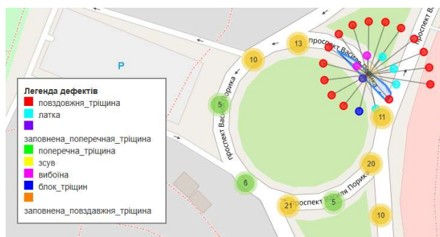
Fig. 3. Example of a defect location map for a road section in an urban area (Vynohradar district, Kyiv)
