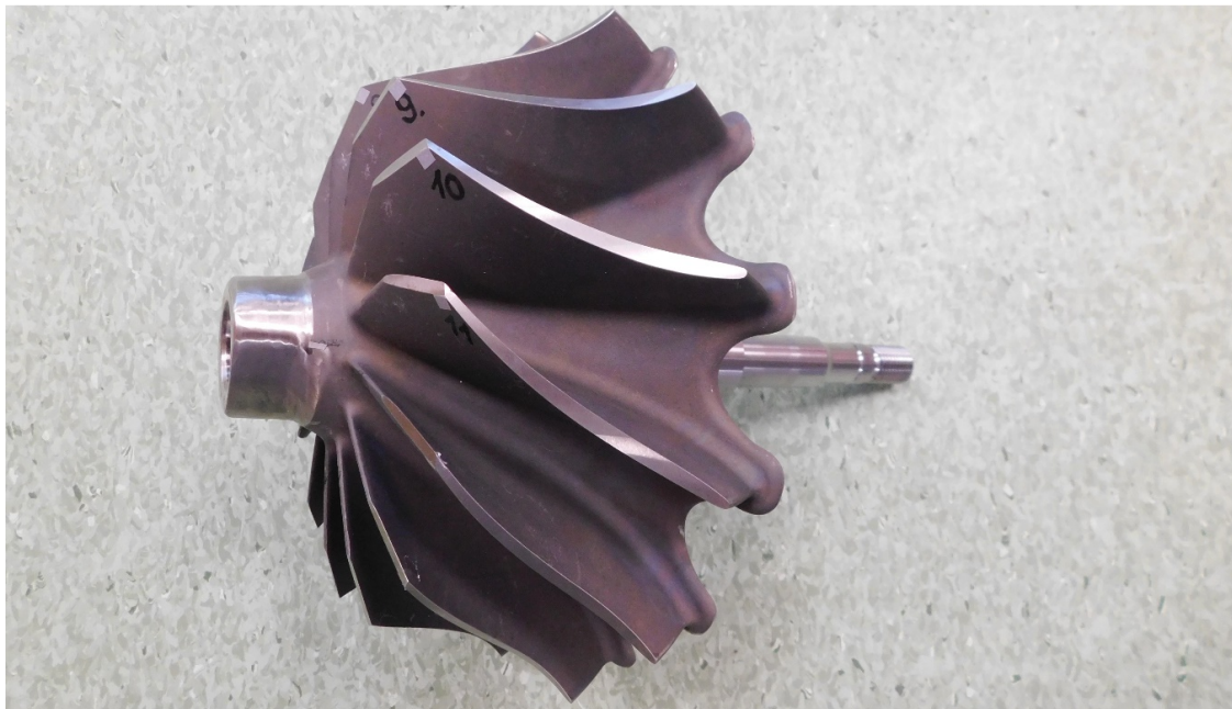
Figure 1. Marine engine turbocharger rotor.
