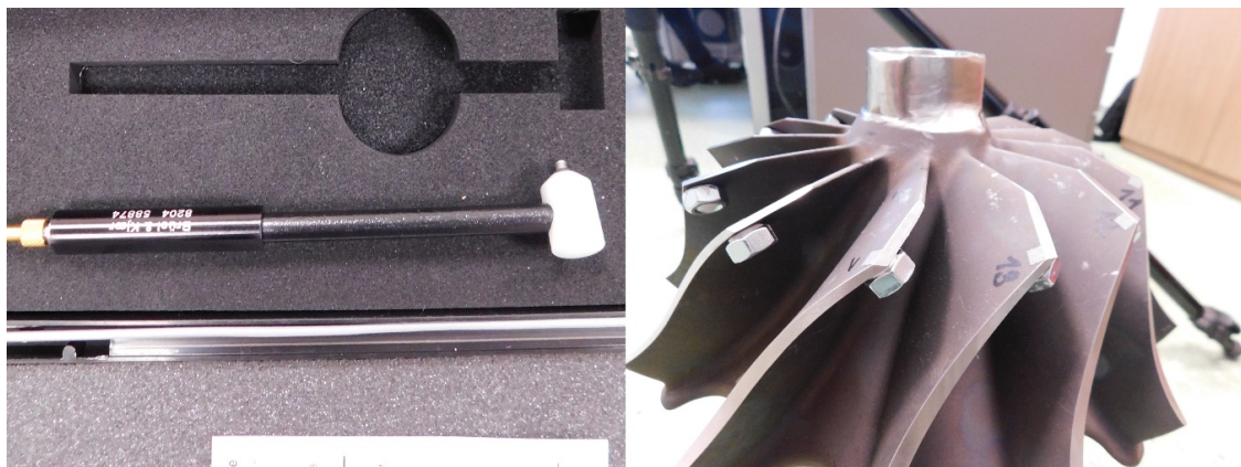
Figure 4. Turbocharger turbine wheel with additional masses on blades and the used modal hammer.
