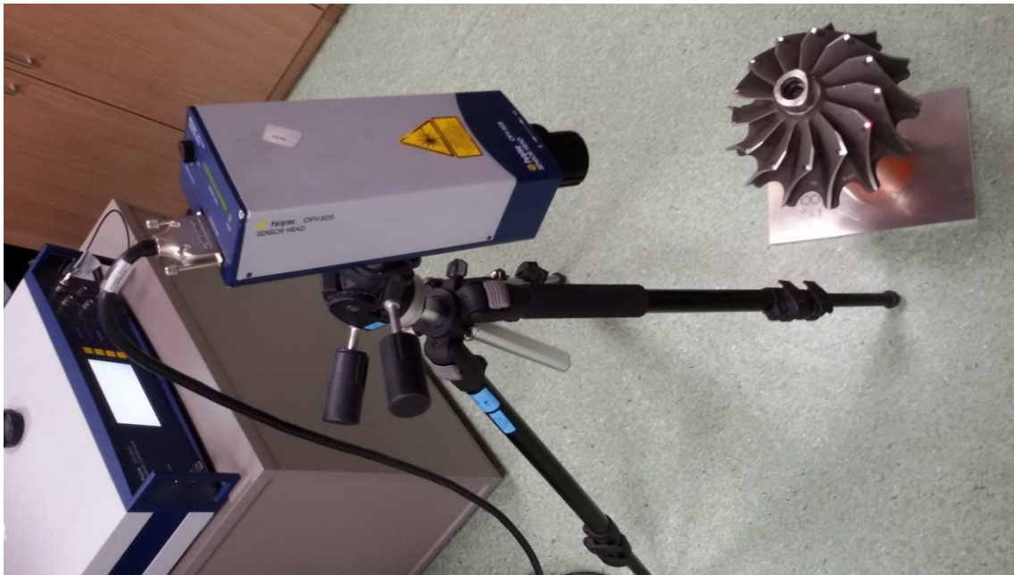
Figure 3. Laser equipment for blade vibration measurement.
