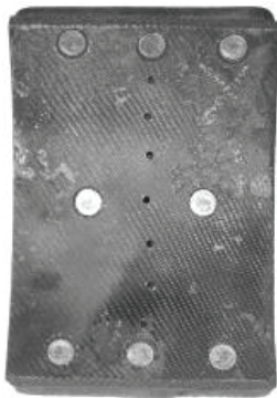
Fig. 5 Thermocouples placing on the working surface of the brake pad
