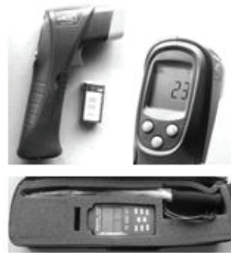
Fig. 6 Measuring equipment. Pyrometer, anemometer
