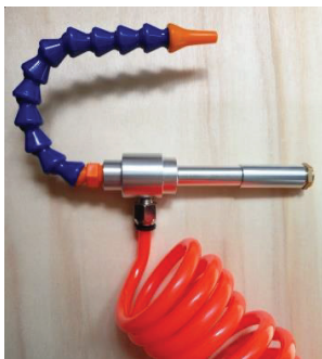
Fig. 3 General view of the Ranque-Hilsch vortex tube
