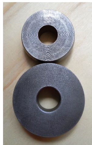
Fig. 7 Friction pair “Disc-Disk”
